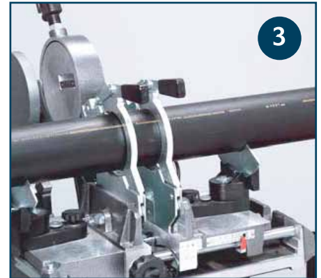
3. Check that the pipe ends match precisely. If necessary clamp and trim again.
