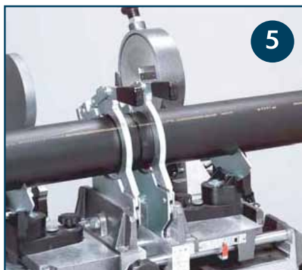
5. Quickly remove the hot plate and slowly increase the welding pressure (see the table on the machine for the welding pressure).
