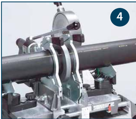
4. Press the pipe ends against the hot plate by briefly applying a high pressure. Continue heating with very low pressure until an upstand of 1 mm has formed.
